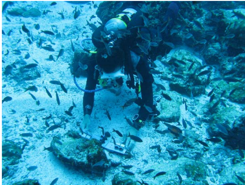
Fig. 8. Onset HOBOT- Pendant light /temperature data logger set deployment with four data loggers to monitor yellow, green, blue and full visible spectrum intensity (lux).
