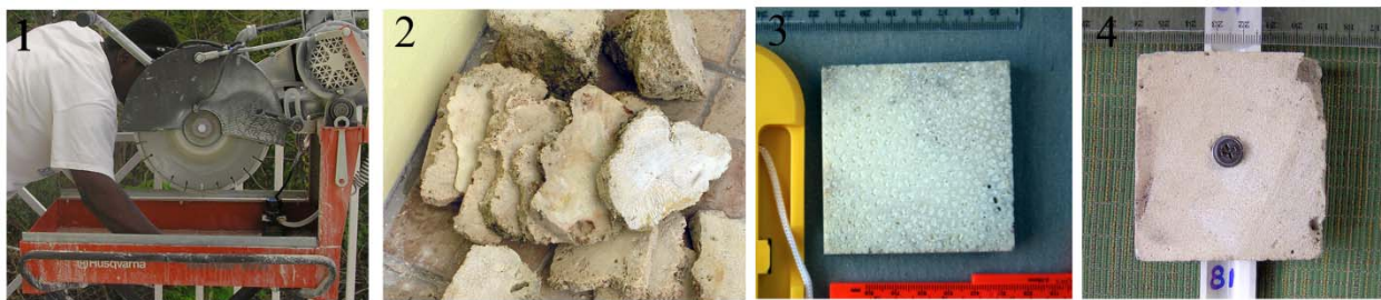
Fig. 14. (1) Masonry saw used to cut the coral fragments, (2) transversal sections of the coral fragments, (3) tile photographed with a size reference, (4) tile attached to the PVC rack for preconditioning.
