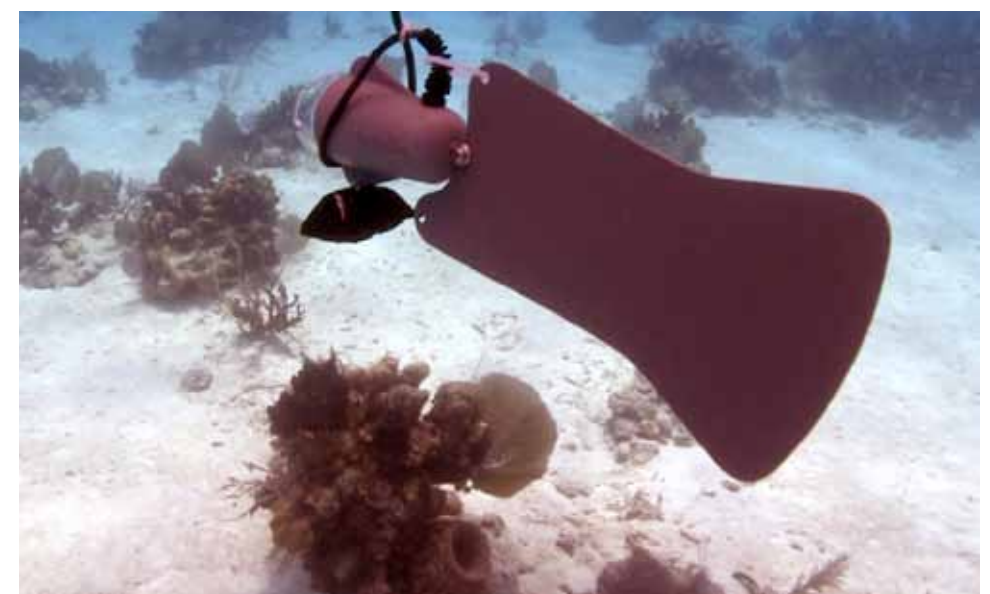
SeaViewer tethered video camera used to characterize habitats.
