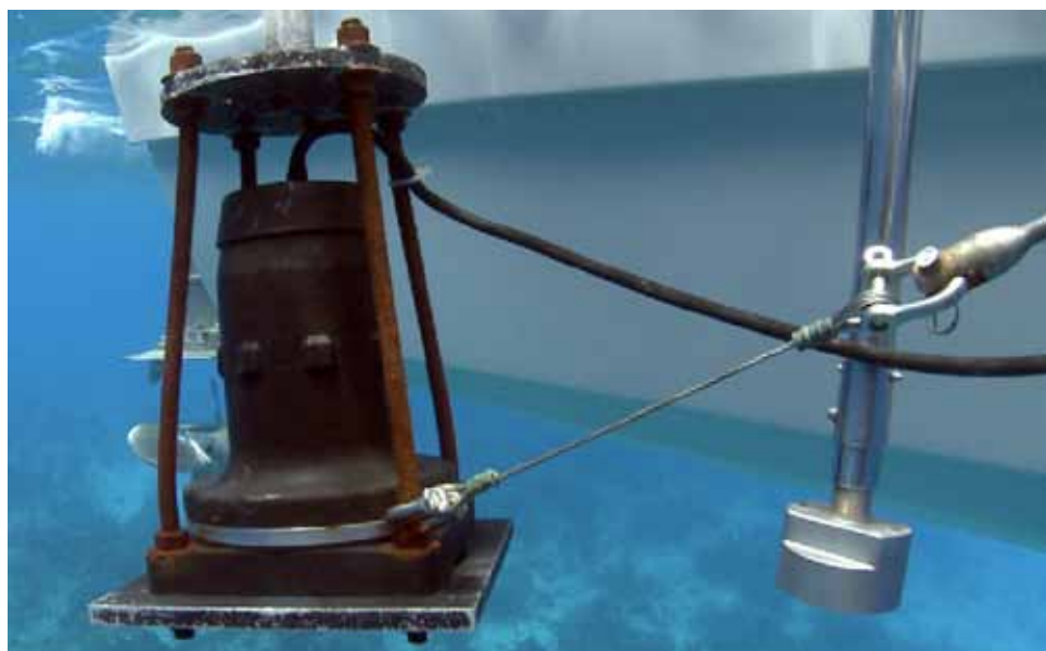
Acoustic sub-bottom profiler (left) and acoustic depth sounder (right) deployed from survey vessel's side. For the sub-bottom profile, a cable transmits data to a laptop aboard the boat while a second cable stabilizes the transducer during travel along the transect line. The cable for the acoustic depth sounder is housed within the metal pipe that attaches it to the boat.
