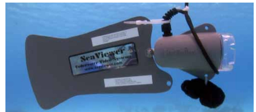
SeaViewer tethered video camera used to characterize habitats.
