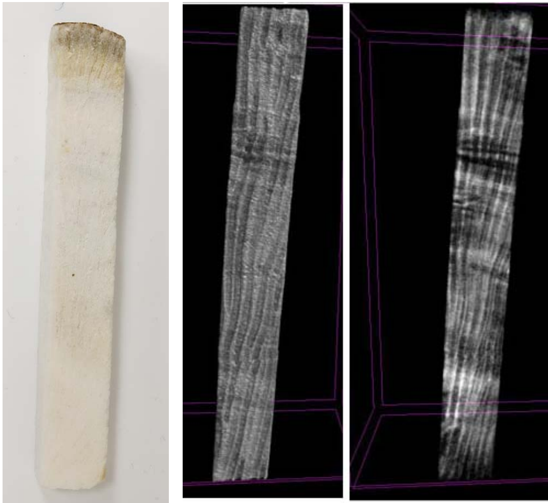
Fig. 10. Cores taken from Porites lobata . Unprocessed core (left), CT scan of the core (center), and CT of a section of the core (right).
